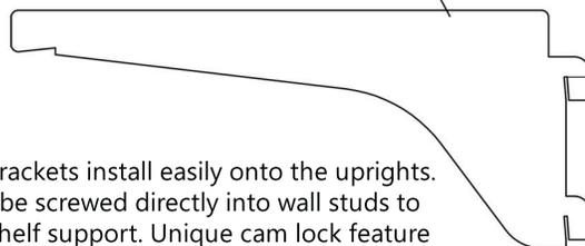
The adjustable brackets install easily onto the uprights. Uprights should be screwed directly into wall studs to provide proper shelf support. Unique cam lock feature keeps the bracket firmly in place.
